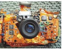
Tightly assembled electronic packages, where electrical connections are required in 3 axes, such as cameras (static application).
